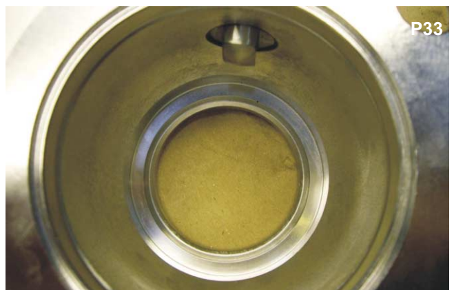
Ensure the valve body is clean and free from any damage.
