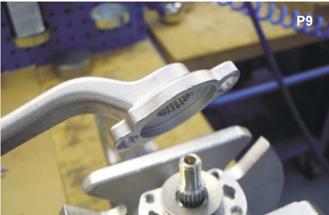
Remove the valve handle.
