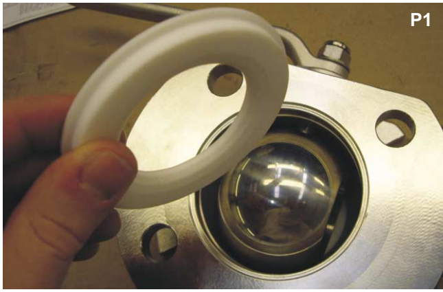
Remove the front ball seal from the valve body.
