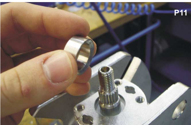
Remove the stuffing collar.
