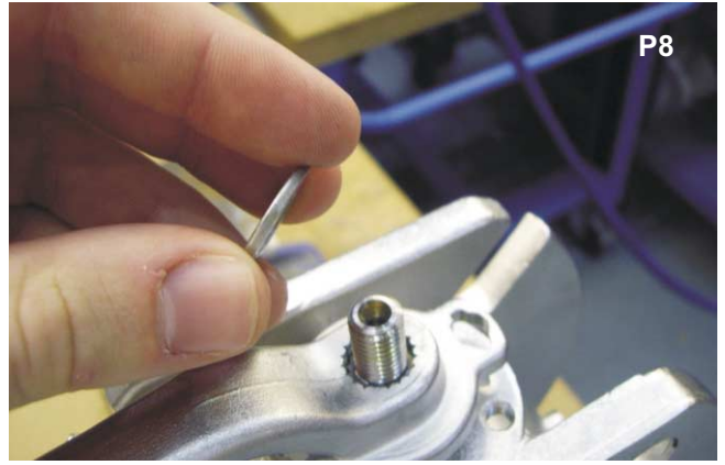
Remove the M10 plain washer.
