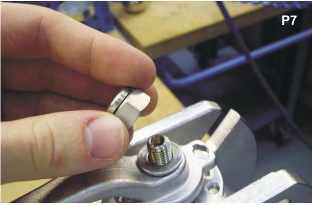
Remove the Lock nut.
