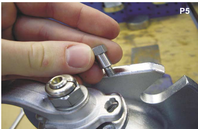
Completely remove the handle stop pin.
