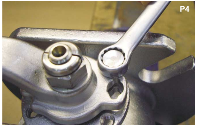
Using a 10mm A/F wrench, remove the handle stop pin.
